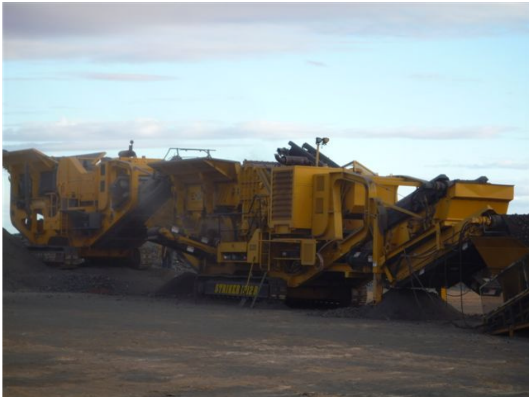
Figure 1: Exact Mining Services – Mobile Primary and Secondary Crushing Units
